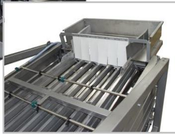
Grading is possible within 4 to 5 size ranges. In order to prevent the fish from accumulating or lying in a transverse position, guide rails with
